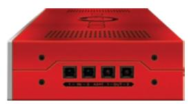
four on the front panel and a further eight on the rear. The four front panel inputs can also operate as unbalanced high impedance inputs for instrument DIs, and analogue inserts (TRS jack) are provided for inputs 1 and 2. The remaining 8 analogue inputs are balanced line level only, and are provided on a DB25 connector on the rear. A further DB25 gives eight balanced line level outputs.
